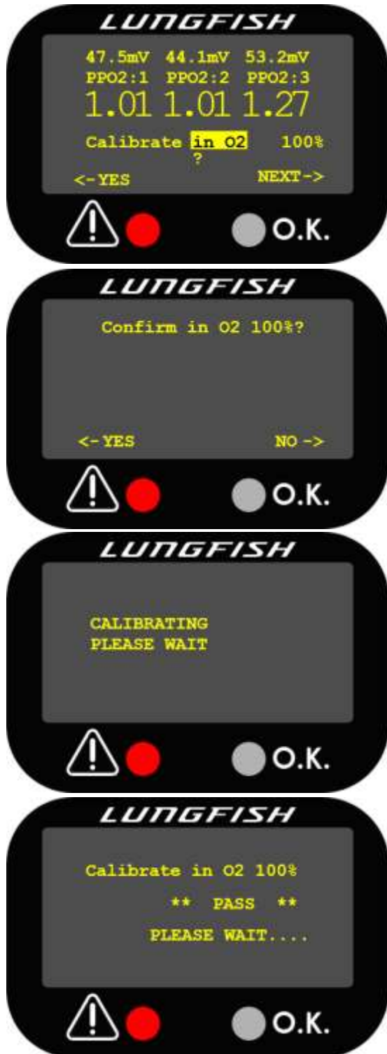
Example of calibration with a changed sensor (Sensor 3)
