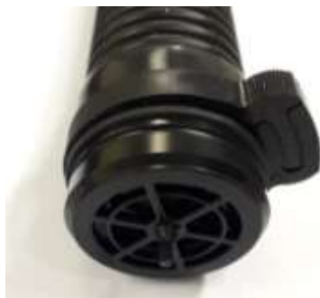
Exhale Hose. Above: Mouthpiece end showing the mushroom valve stem. Below: Exhale Counterlung connection.
